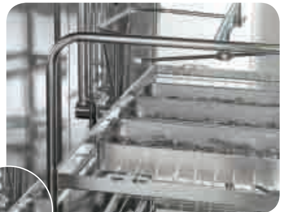
Integrated manifold recognizes that instrument rack has been loaded.
